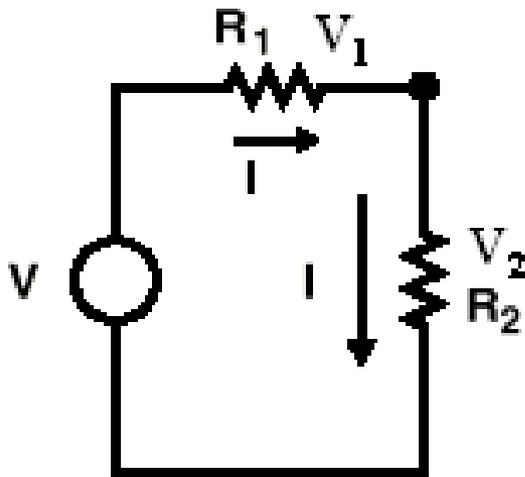
$$V_2 = \frac{R_2}{R_1 + R_2} V$$
